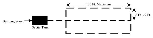
A gravel system must be looped together
