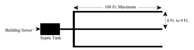
A gravelless or chamber system is not looped together
